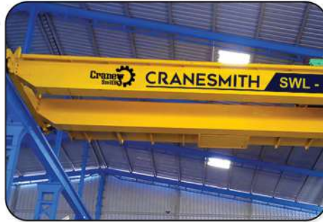
Double Girder EOT Crane
